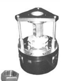
This chuck is used for centrifugally casting of Caterpillar® heavy equipment brake drums. It is designed to hold multiple diameter parts, ranging from 25.9" to 35.35" at a maximum of 400 R.P.M. It also can withstand temperatures in excess of 800 degrees Fahrenheit. Non-magnetic Stainless Steel is used to minimize the conducted heat away from the chuck at the six contact points of the drum. Optional copper shielding can also be used to deflect
