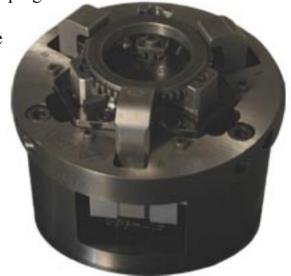
Market pressures combined with advances in CNC equipment and better inserts and coatings have driven speeds and feeds to extreme levels. Pullback chucks help the efficiencies of lathe turning by reducing clamping force requirements, while minimizing centrifugal force effects
