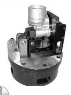
This chuck was designed to be able to accommodate different parts. Simple and quick tooling setup. Doubled throughput. Reduced scrap rate from 5% to 0%. Positive quick loading.
