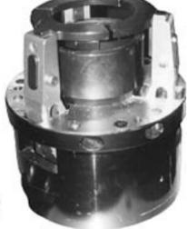
This chuck was designed to be able to accommodate different parts. Simple and quick tooling setup. Doubled throughput. Reduced scrap rate from 5% to 0%. Positive quick loading.
